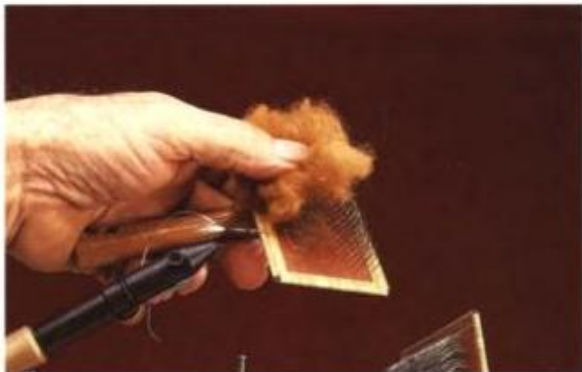
3. Place a small amount of wool on one of the brushes. Place the other brush on top, forming a wool sandwich. Press the brushes together, then pull them in opposite directions, allowing the wires to pull the wool fibers apart.
